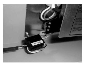
Open the bead by gently prying the latch with a thumbnail or small screwdriver. Loop the wiring as shown, then place the bead over the wires and gently squeeze shut until the latch snaps shut, indicating that the cable has been correctly covered.
