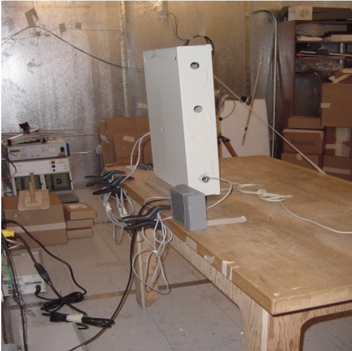
(BVCACDRM-13M) Conducted Emissions Set-Up
