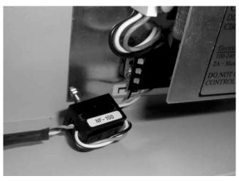
Open the bead by gently prying the latch with a thumbnail or small screwdriver. Loop the wiring as shown, then place the bead over the wires and gently squeeze shut until the latch snaps shut, indicating that the cable has been correctly covered.
