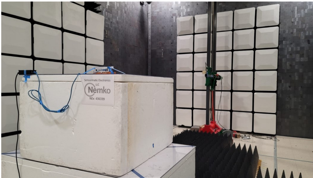
Figure 6 - Radiated emissions above 1 GHz (18 – 26 GHz), rear view, 3 meters distance.
