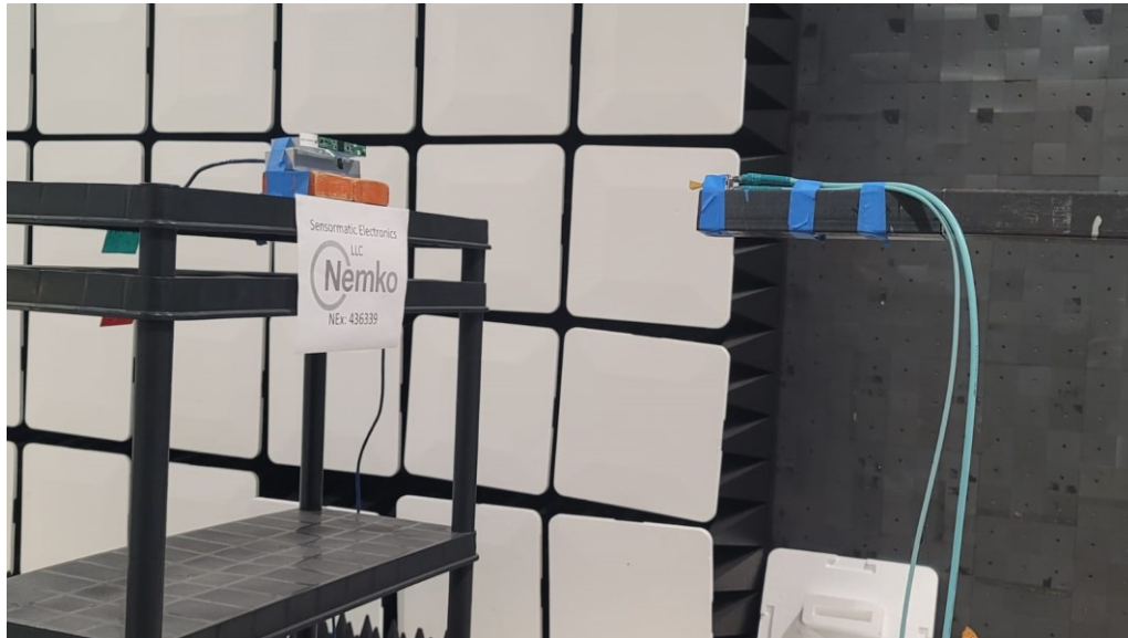
Figure 13 - Radiated emissions above 1 GHz (110 – 200 GHz), front view, 0.4 meters distance.
