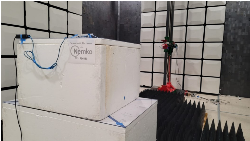
Figure 4 - Radiated emissions above 1 GHz (1 – 18 GHz), rear view, 3 meters distance.
