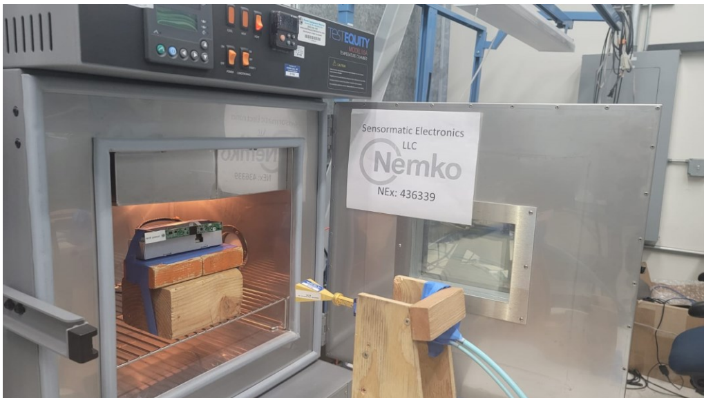
Figure 18 – Frequency stability test setup.
