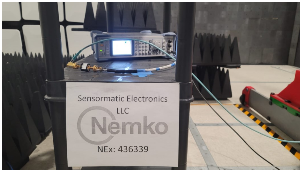
Figure 16 – Test setup (conducted test).
