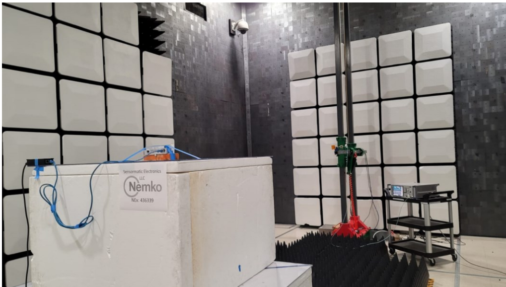
Figure 8 - Radiated emissions above 1 GHz (26 – 40 GHz), rear view, 3 meters distance.
