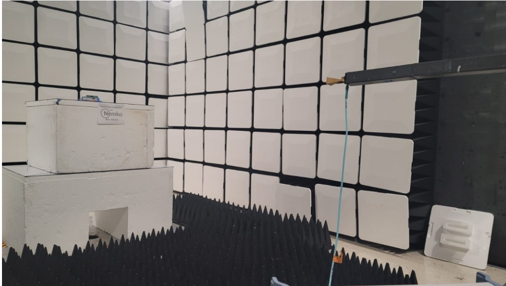
Figure 9 - Radiated emissions above 1 GHz (40 – 50 GHz), front view, 3 meters distance.
