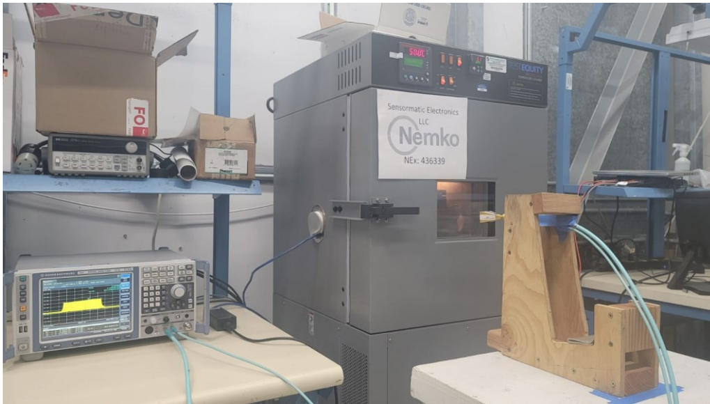
Figure 17 – Frequency stability test setup.
