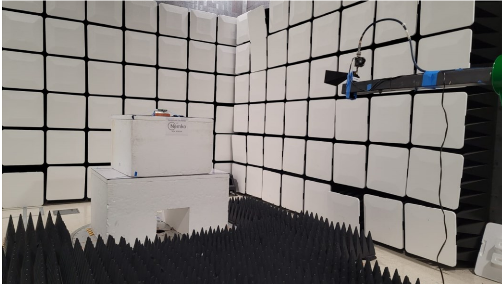
Figure 5 - Radiated emissions above 1 GHz (18 – 26 GHz), front view, 3 meters distance.
