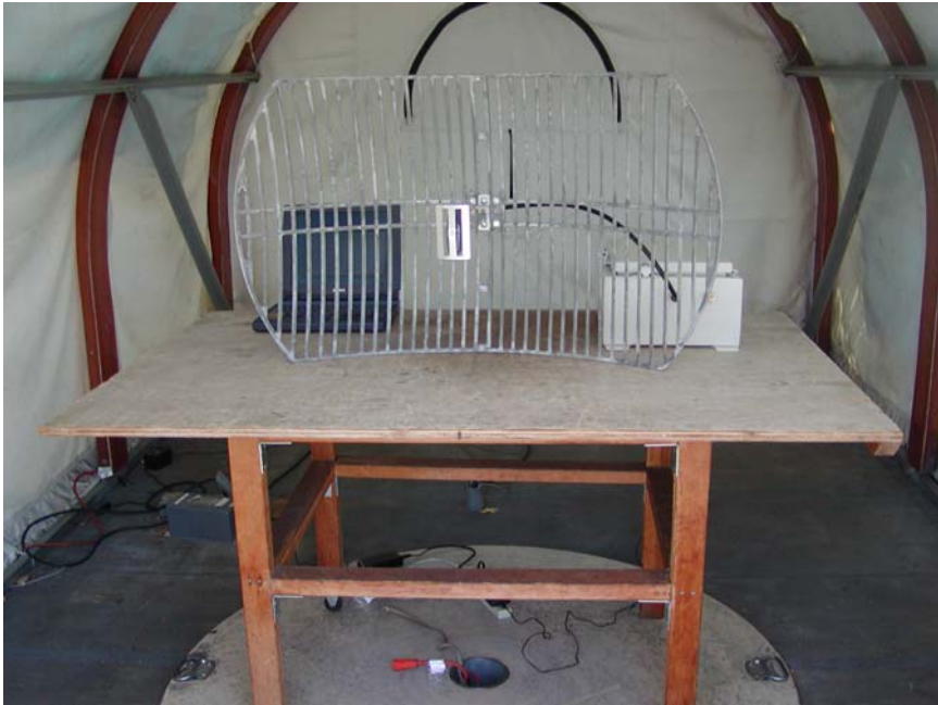
Radiated Emission with 24dBi Dish Antenna - Front View
