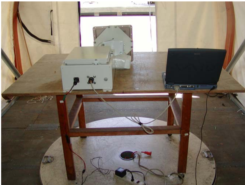
Radiated Emission with 16dBi Patch Antenna – Rear View
