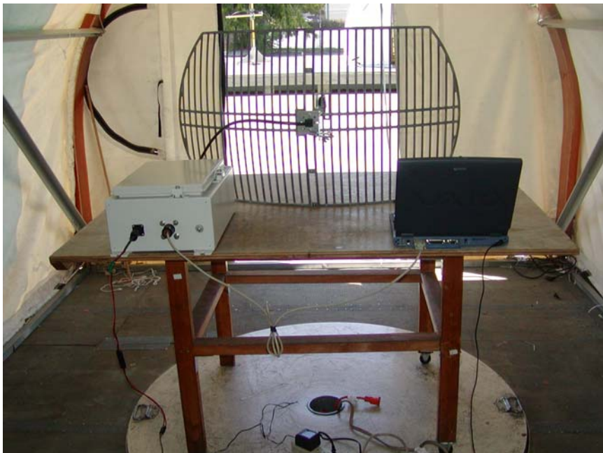
Radiated Emission with 24dBi Dish Antenna - Rear View
