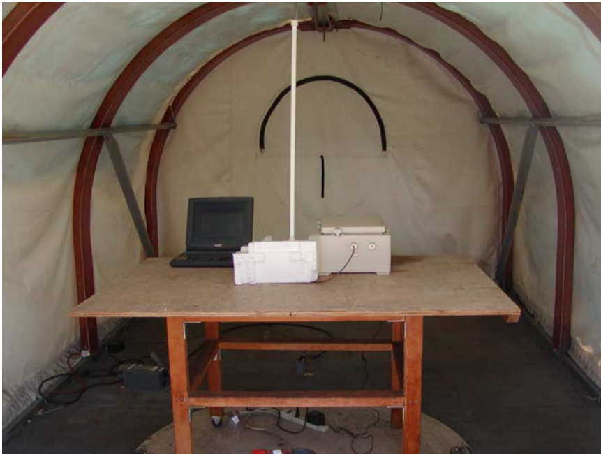
Radiated Emission with 10dBi Whip Antenna – Front View
