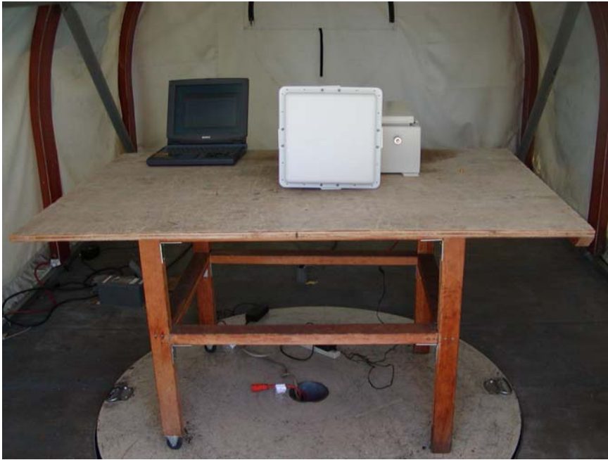
Radiated Emission with 16dBi Patch Antenna – Front View
