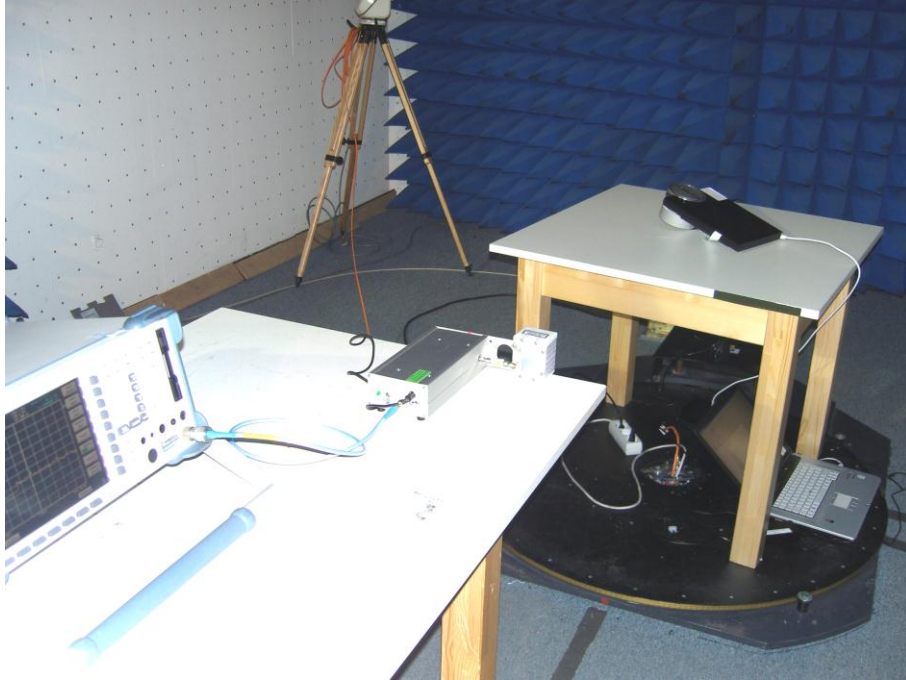
Anechoic chamber (Test setup for 30 GHz – 40 GHz)
