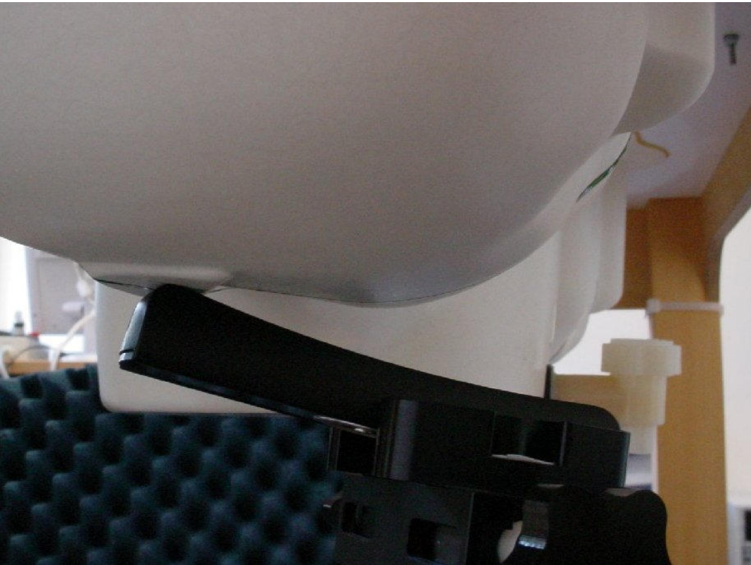
Photo 14: Test position right hand tilted 15°
