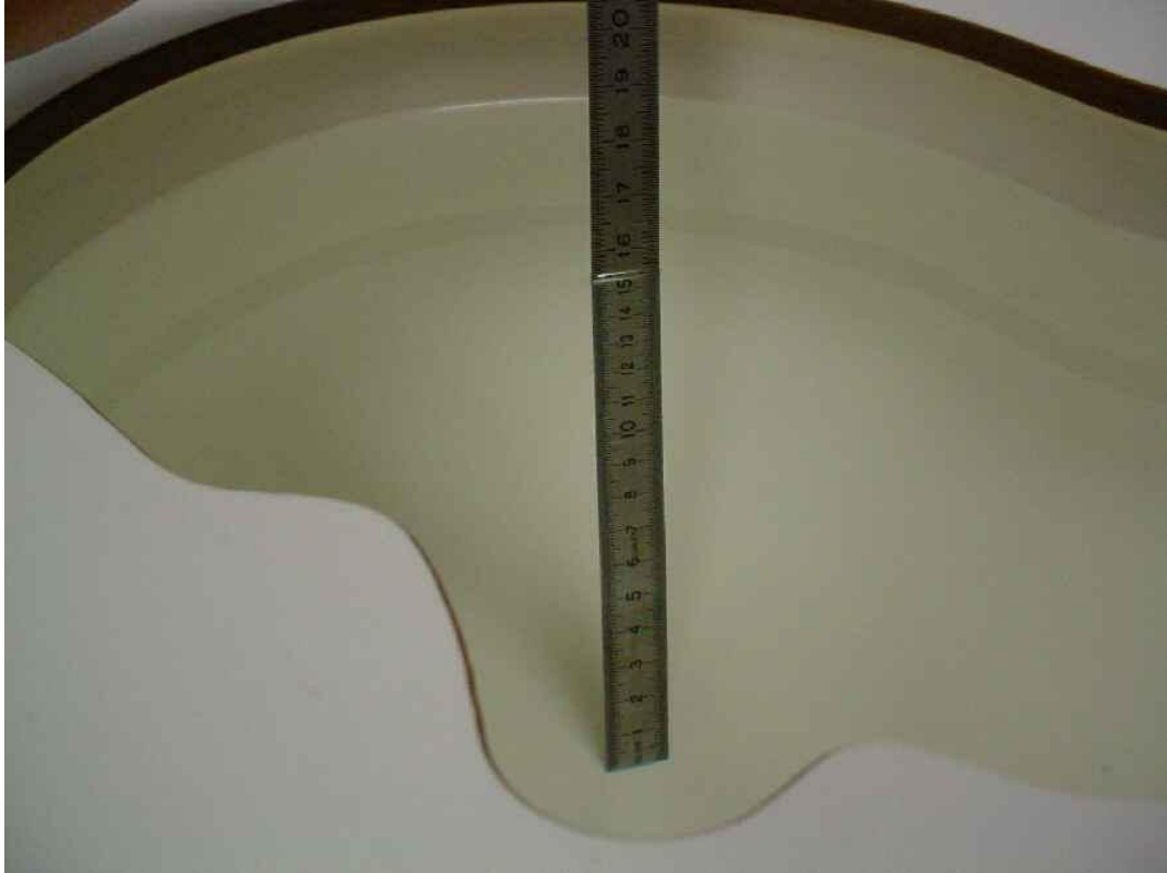
Photo 20: Liquid depth 1900 MHz body simulating liquid
