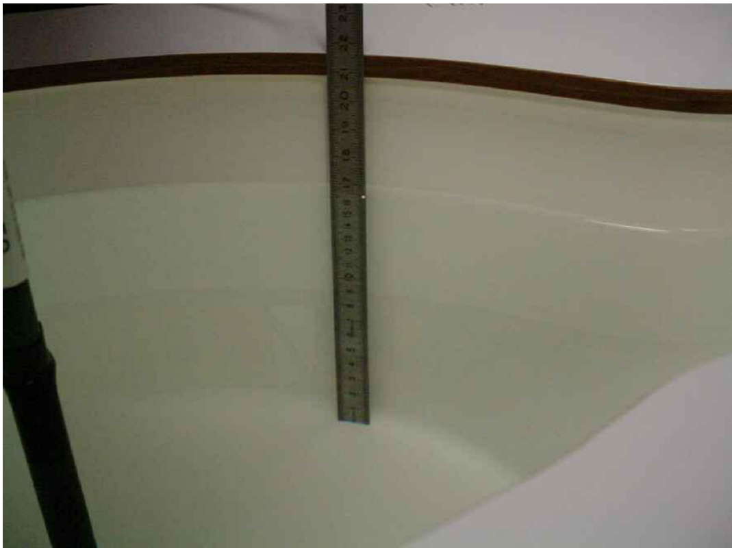
Photo 20: Liquid depth 1900 MHz body simulating liquid
