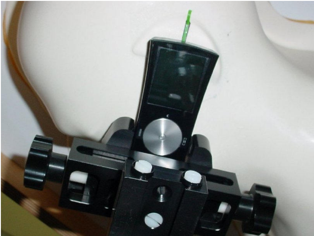
Photo 8: Test position left hand tilted 15°
