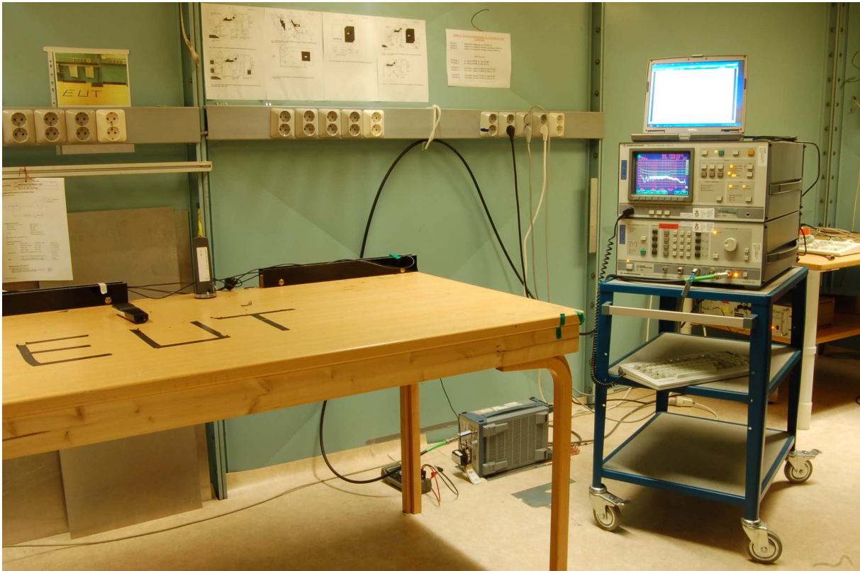
Power line Conducted Emissions Test
