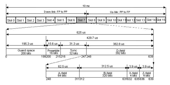
The basic, repeating, frame structure is 10 ms long. It is sub-divided into 16 slots, each 625  $\mu$ s long. The active transmission time is 429.7  $\mu$ s. The first 8 slots form the 'down-link', when the FP transmits to the PPs. The last 8 slots form the 'up-link', when the PPs transmit to the FP.
