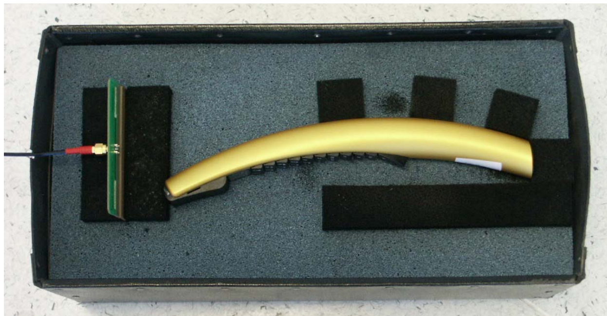
Fig. 8: Provide testbox to control the output power.
