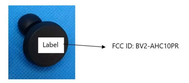
Note: The device is impracticable to label with a font size that is four points or larger, the FCC ID will be placed in the user manual, and the FCC ID will also be placed on a removable label attached to the device.
