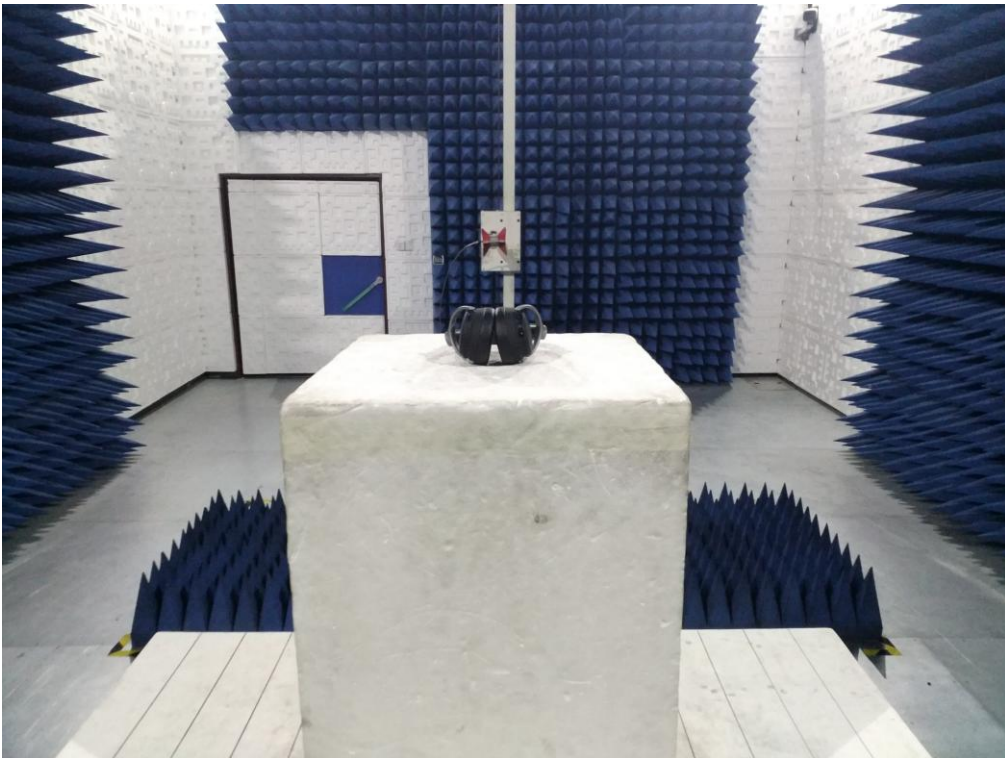
RADIATED EMISSION TEST SETUP ABOVE 1GHZ
