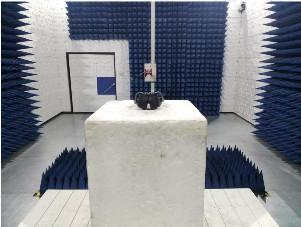
RADIATED EMISSION TEST SETUP ABOVE 1GHZ
