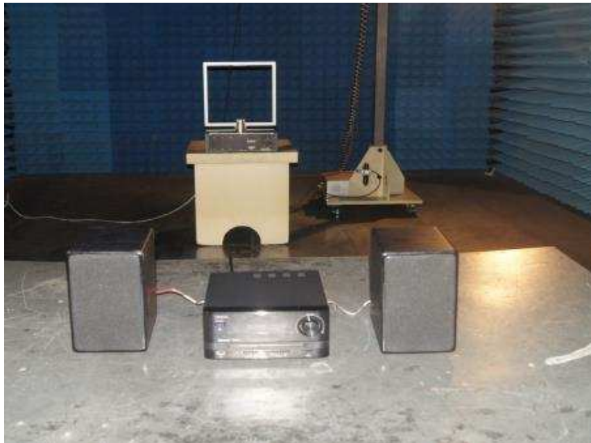
Photograph 2: Set-up for Radiated Spurious Emissions (30MHz-1GHz)
