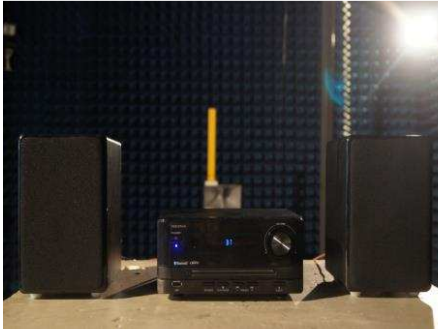
Photograph 4: Set-up for Radiated Spurious Emissions (18GHz ~ 26GHz)
