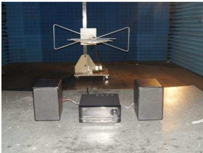
Photograph 2: Set-up for Radiated Spurious Emissions (30MHz-1GHz)
