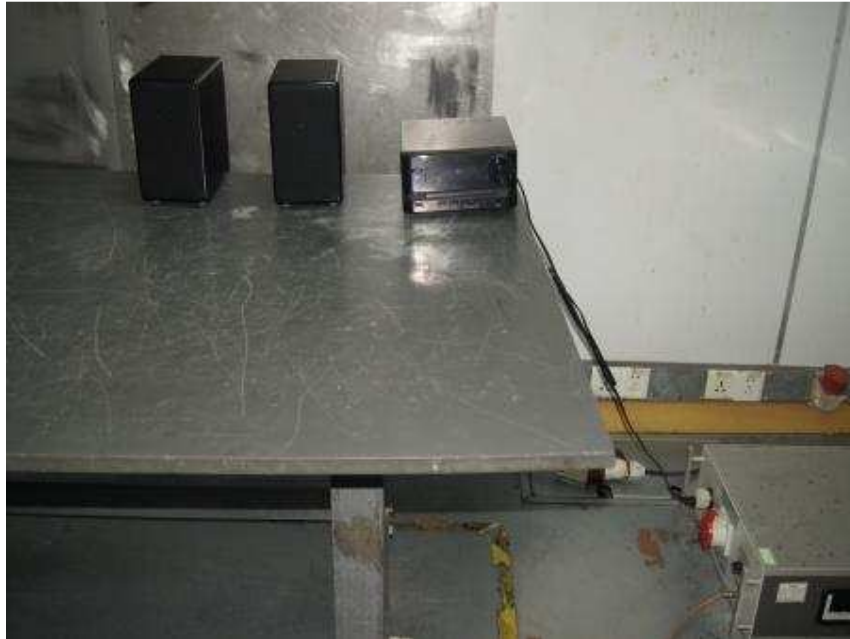
Photograph 5: Set-up for Conducted Emissions
