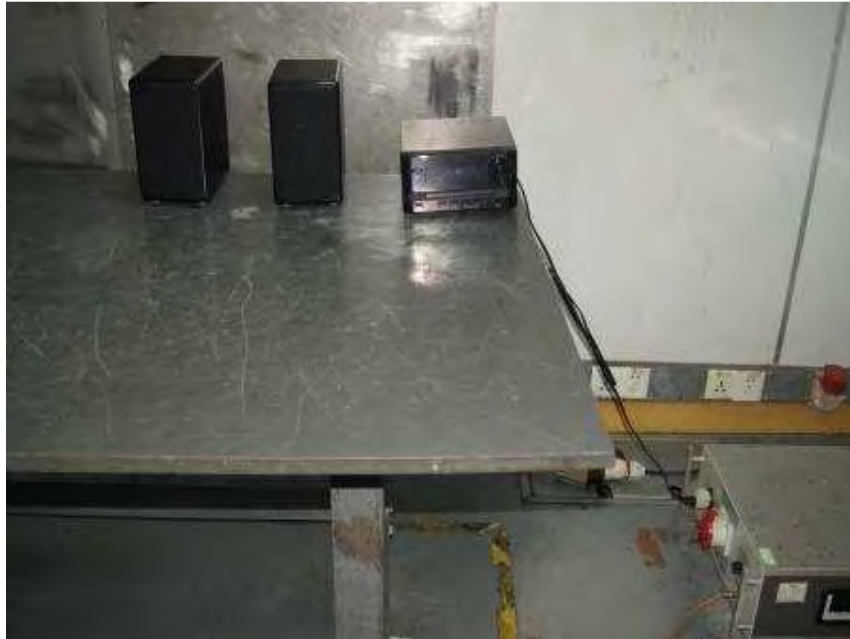
Photograph 5: Set-up for Conducted Emissions
