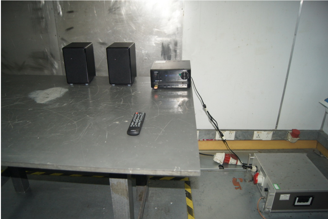
Photograph 6: Set-up for Radiated Emissions, below 1GHz
