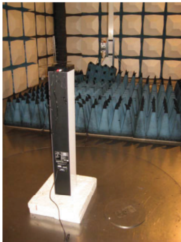
Photograph 3: Set-up for Radiation Measurement above 1GHz
