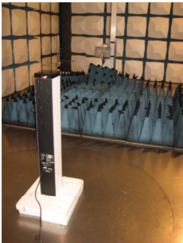
Photograph 3: Set-up for Radiation Measurement above 1GHz
