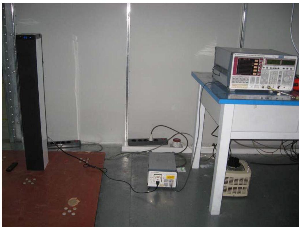
Photograph 1: Set-up for Conducted Emission
