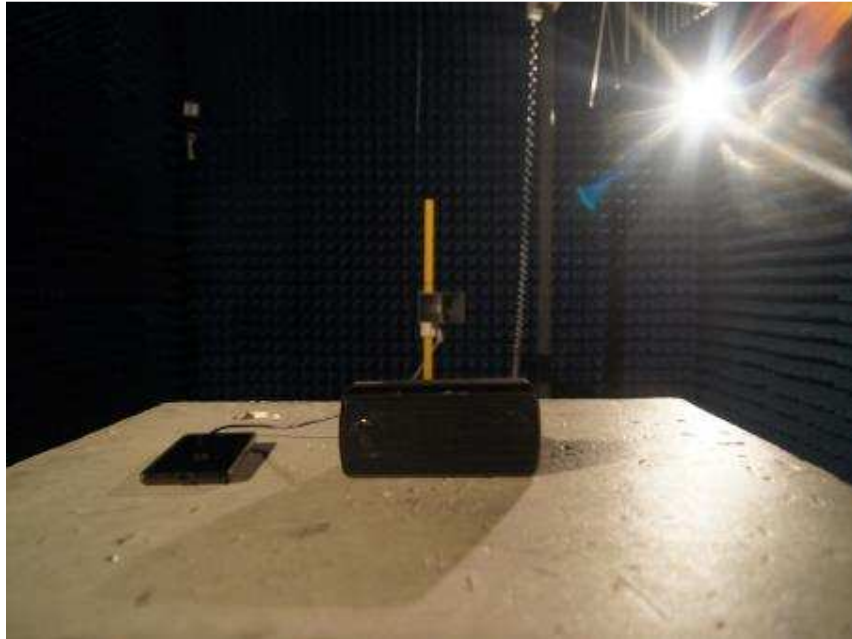
Photograph 4: Set-up for Radiated Spurious Emissions (18GHz ~ 26GHz)
