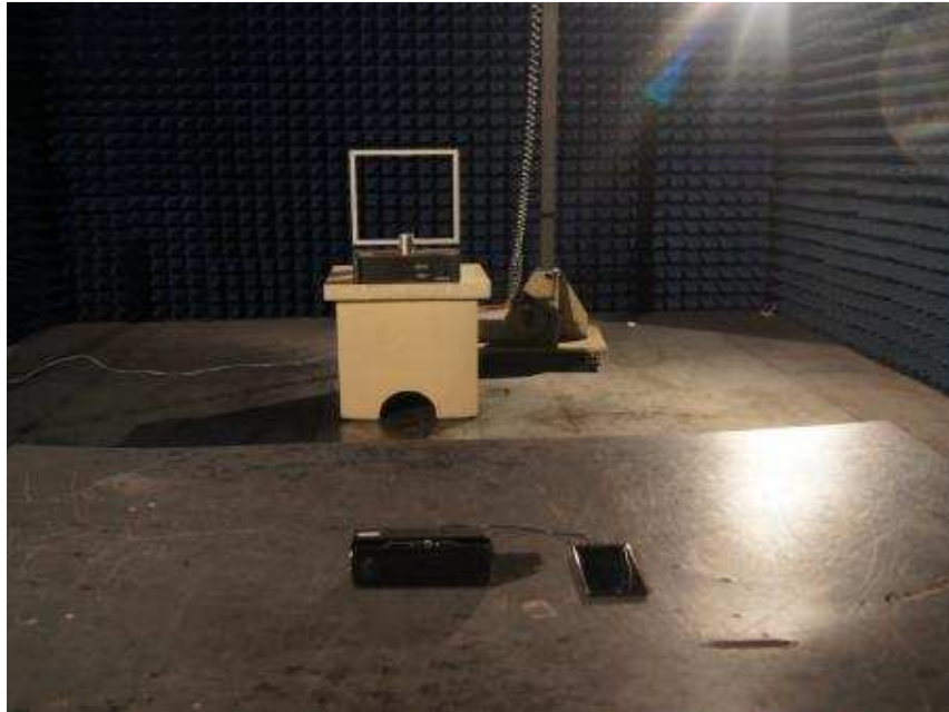
Photograph 2: Set-up for Radiated Spurious Emissions (30MHz-1GHz)
