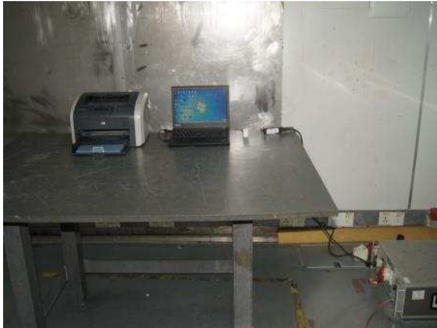
Photograph 5: Set-up for Conducted Emissions
