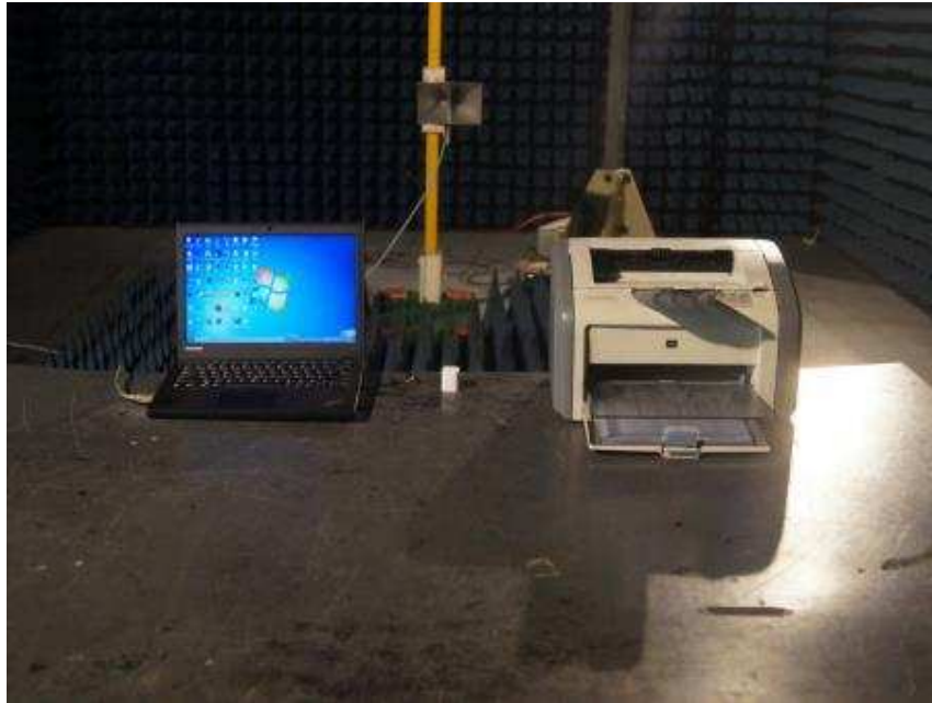
Photograph 7: Set-up for Radiated Emission (Above 1GHz)
