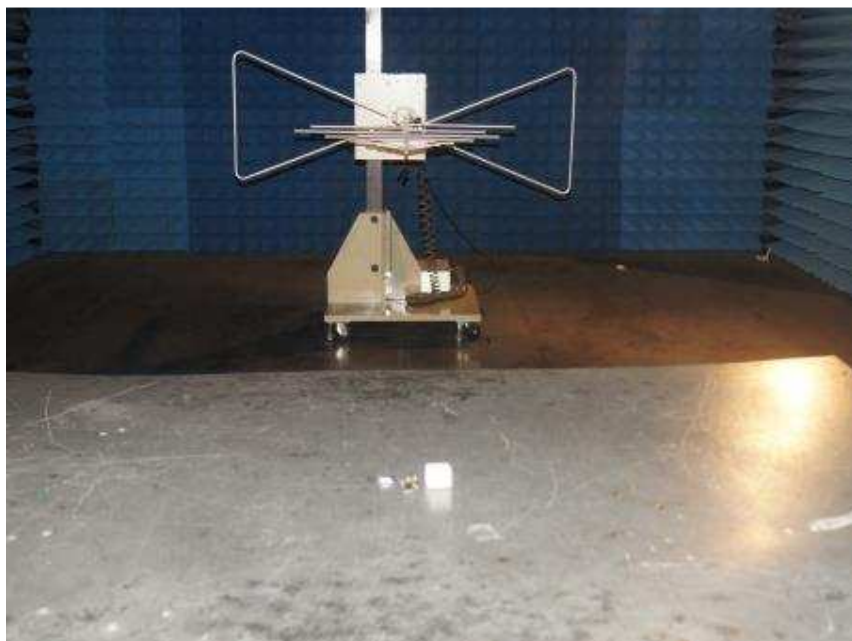
Photograph 2: Set-up for Radiated Spurious Emissions (30MHz-1GHz)
