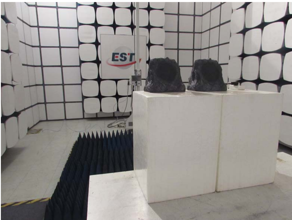
Radiated Test (1000-25000 MHz)
