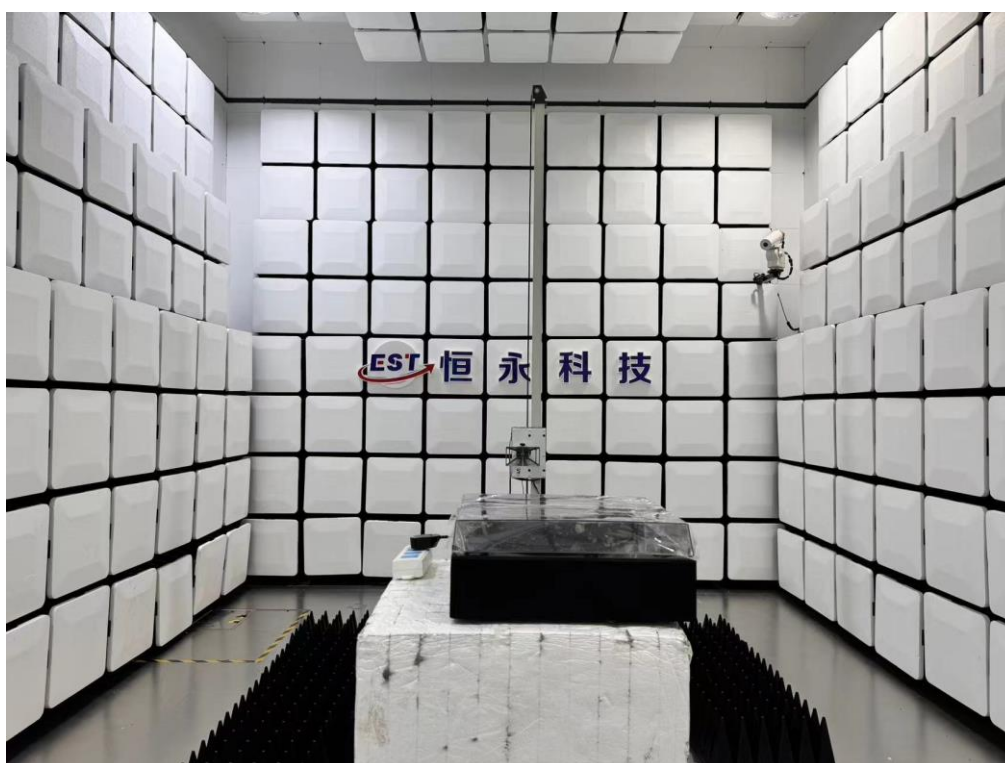
Radiated emission test: Above 1GHz
