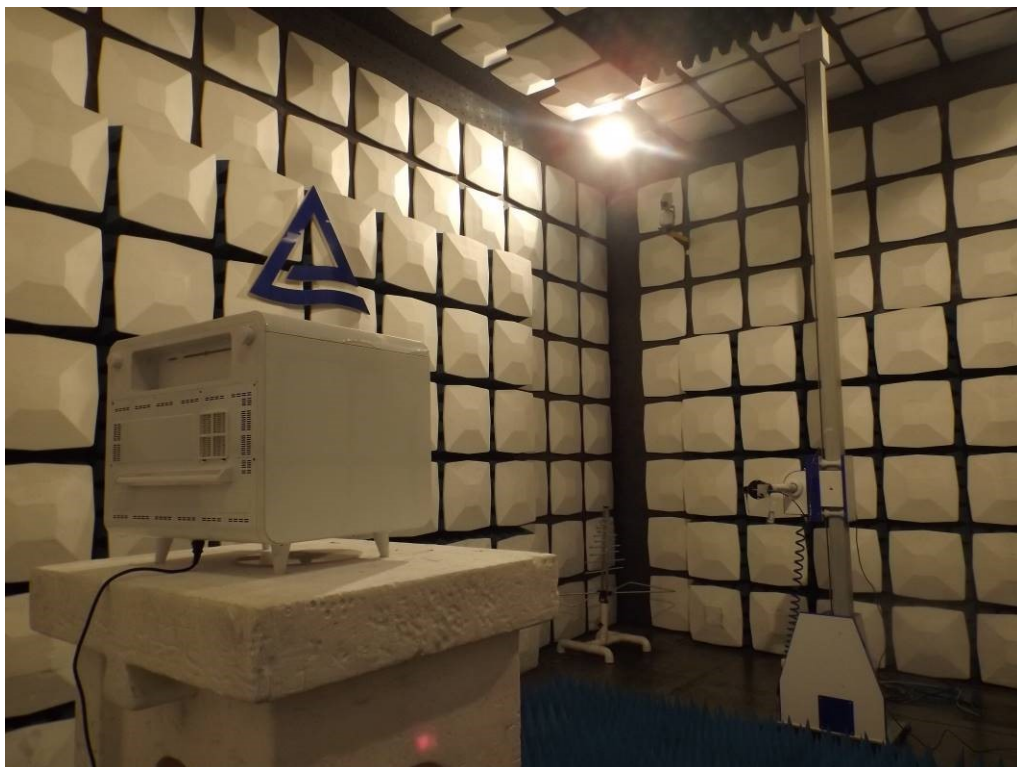
Photograph 4: Set-up for Radiated Spurious Emission, 18GHz - 26.5GHz
