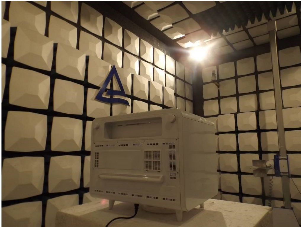
Photograph 4: Set-up for Radiated Spurious Emission, 18GHz - 26.5GHz
