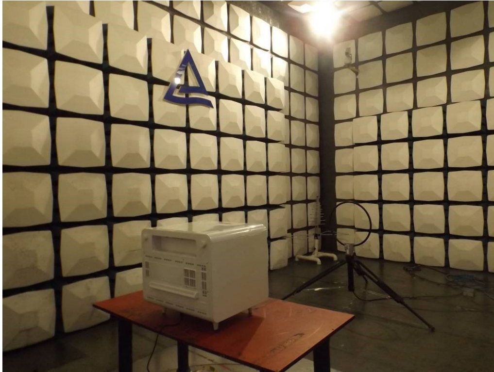
Photograph 2: Set-up for Radiated Spurious Emission, 30MHz - 1GHz
