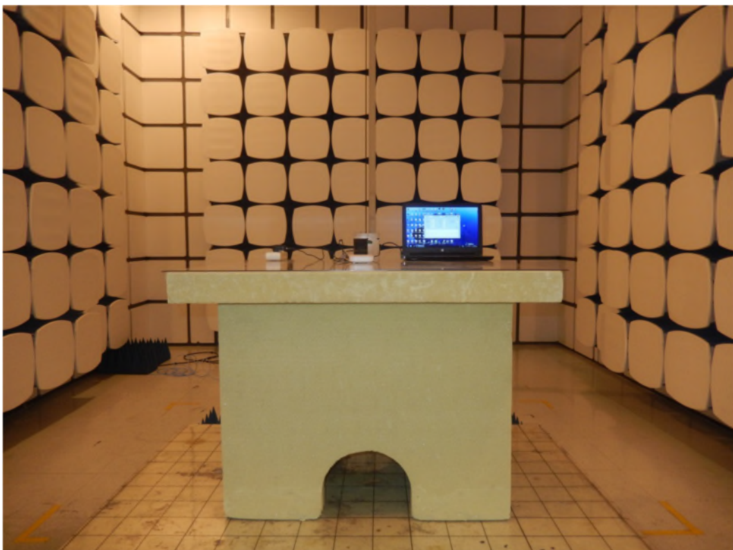
Photograph 2: Set-up for Radiated Spurious Emission, above 1GHz
