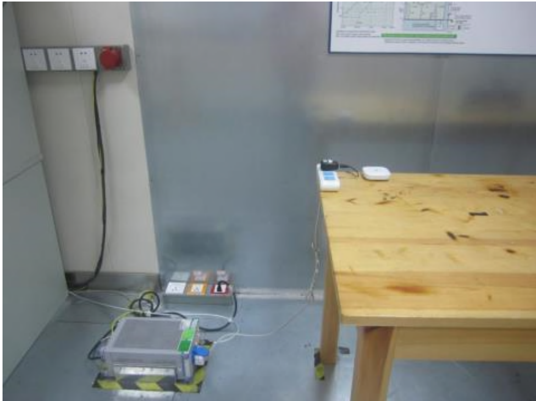
Photograph 3: Set-up for Conducted Emissions
