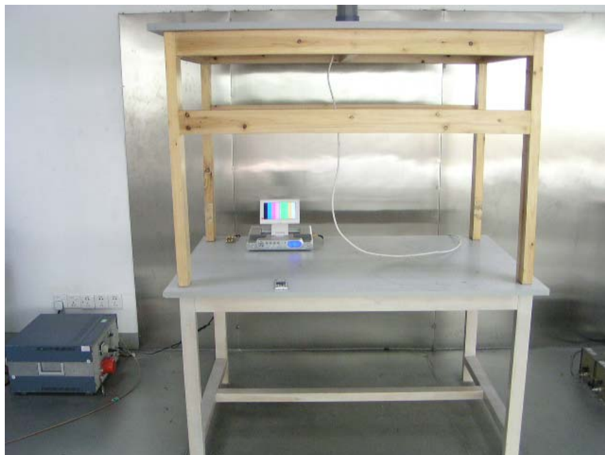
TV Mode: Conducted Emission - Front View
