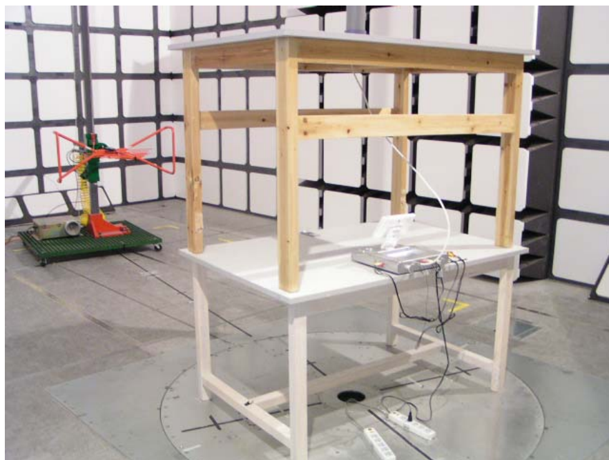
TV Mode: Radiated Emission - Rear View
