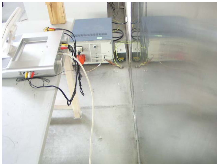
TV Mode: Conducted Emission - Side View
