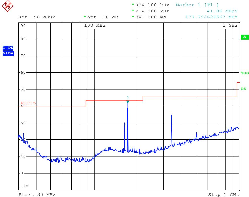
CMA 7" LCD TV &amp; Radio M/N:KCL8806DT Radiation Weather Band
