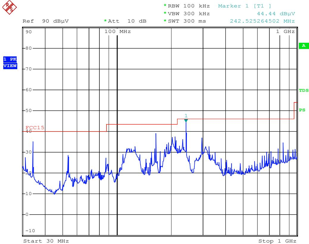
CMA 7" LCD TV & Radio M/N:KCL8806DT Radiation TV Channel 13
