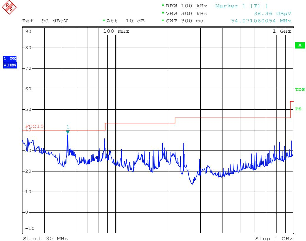
CMA 7" LCD TV & Radio M/N:KCL8806DT Radiation TV Channel 69
