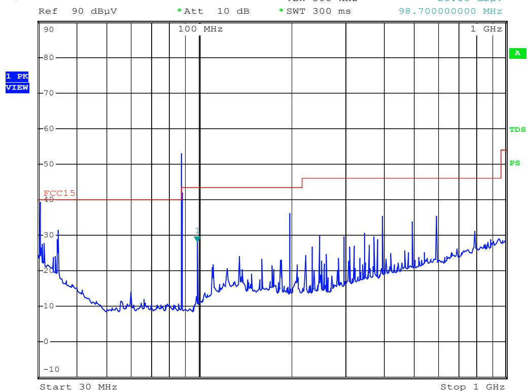
CMA 7" LCD TV & Radio M/N:KCL8806DT Radiation FM88MHz Horizo
