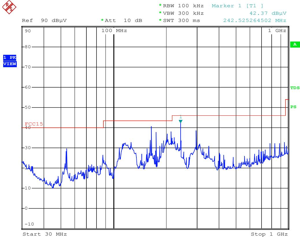
CMA 7" LCD TV &amp; Radio M/N:KCL8806DT Radiation TV Channel 7
