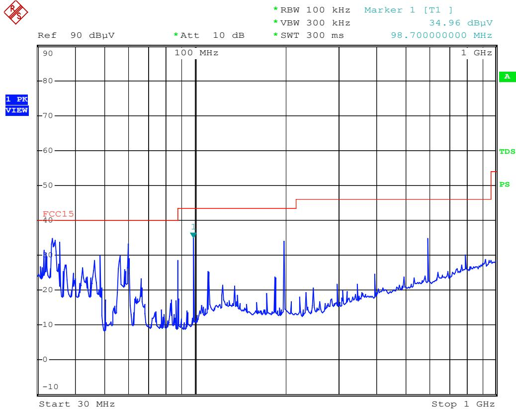
CMA 7" LCD TV & Radio M/N:KCL8806DT Radiation FM88MHz Vertic
