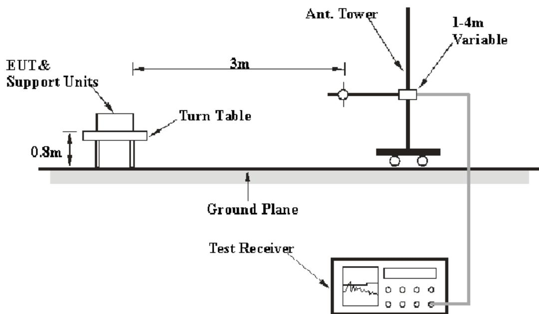
The radiated emission tests were performed in the 3 meters chamber A test site, using the setup accordance with the ANSI C63.4-2003. The specification used was the FCC Part 15 Class B limits.
