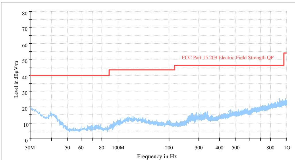
Note: All radiated emissions are 20 dB below the limit or are on the system noise floor level.
