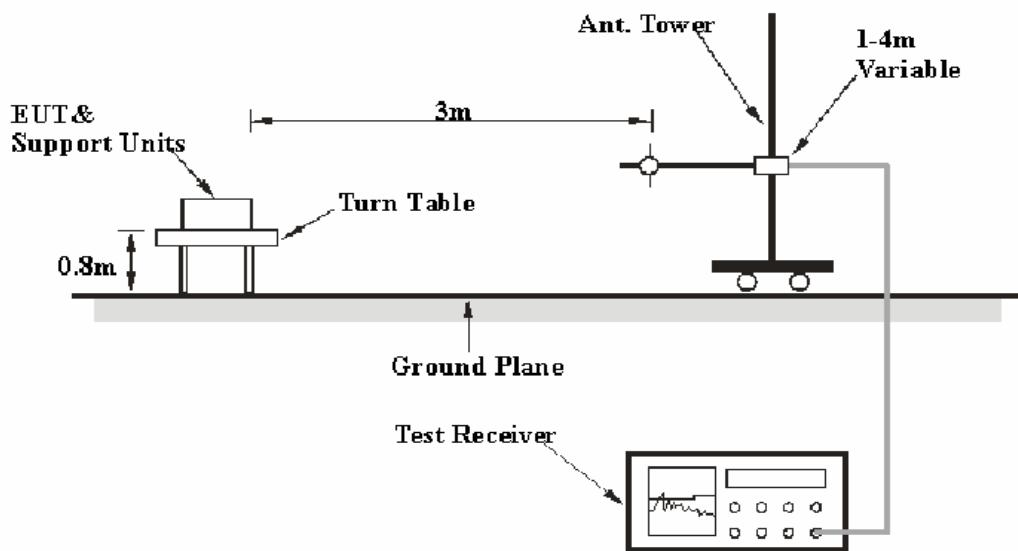
The radiated emission tests were performed in the 3 meters test site, using the setup accordance with the ANSI C63.4-2009. The specification used was the FCC 15.205 and 15.209 limits.
