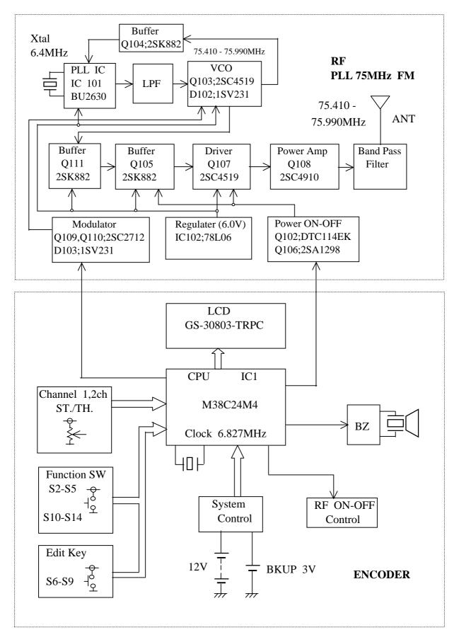
Figure 5.1 Transmitter Block Diagram
