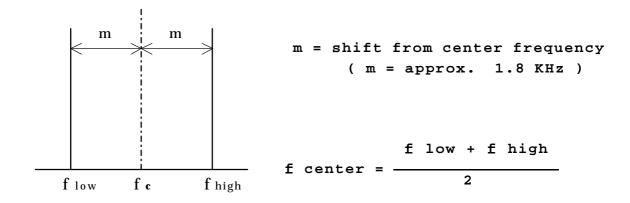
The peak-to-peak deviation of the FSK signal is approximately 3.6 KHz ("sliver modulation")
