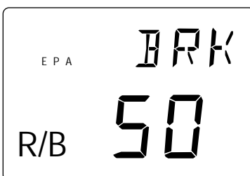
Brake Travel Adjustment (Grip Lever A), (page 25)
