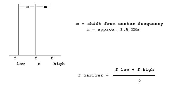
The peak-to-peak deviation of the FSK signal is approximately 3.6 KHz ("sliver modulation")
