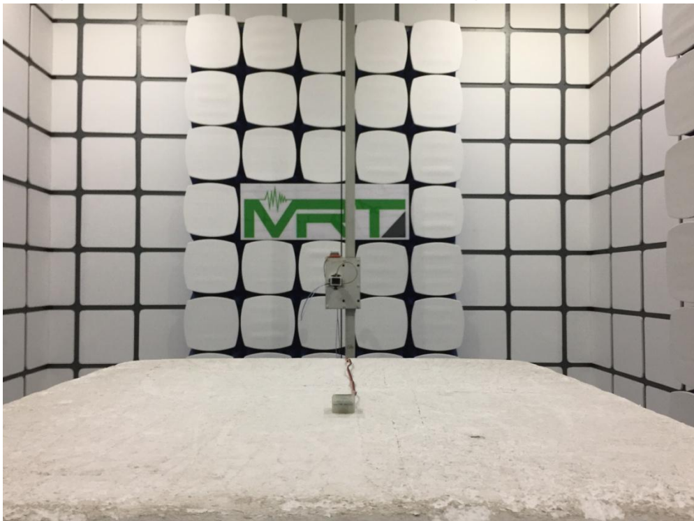
Description: Radiated Spurious Emissions Test Setup for 18 ~ 25GHz
