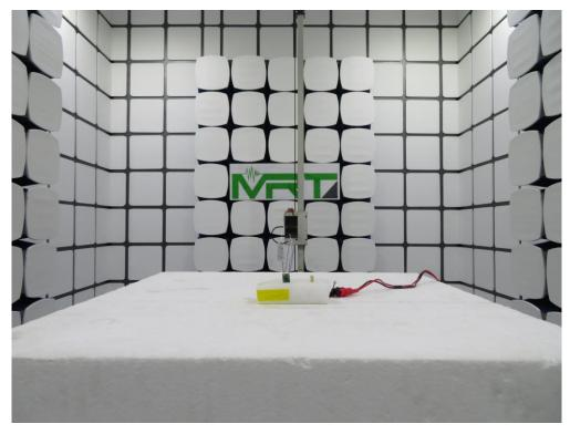
Description: Radiated Spurious Emission Test Setup for 18GHz ~ 25GHz
