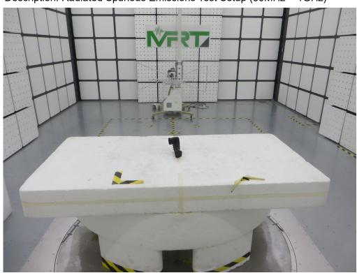
Description: Radiated Spurious Emissions Test Setup (30MHz ~ 1GHz)
