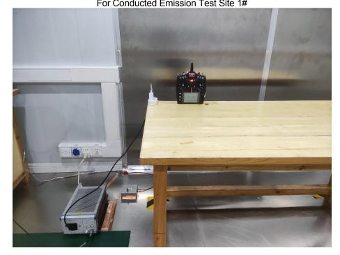
**1.1 Photograph – Conducted Emission Test Setup** For Conducted Emission Test Site 1#
