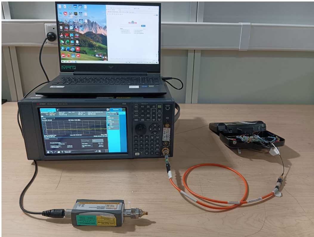
Description: Conducted Test Setup
