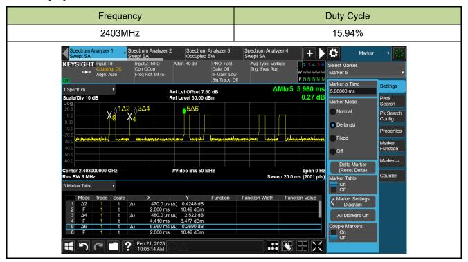
Duty cycle is fixed by software and cannot be changed, declared by the manufacturer. The device is a source-based controlled device. Refer to operation description.
