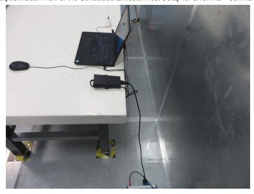
Description: Radiated Emission Test Setup for 9kHz ~ 30MHz (SPM9745) (0.8m Height)
