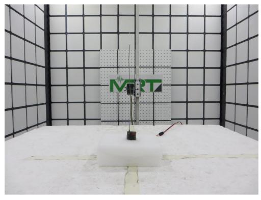
Description: Radiated Emission Test Setup for 18GHz ~ 25GHz (SPM9746) (1.5m Height)
