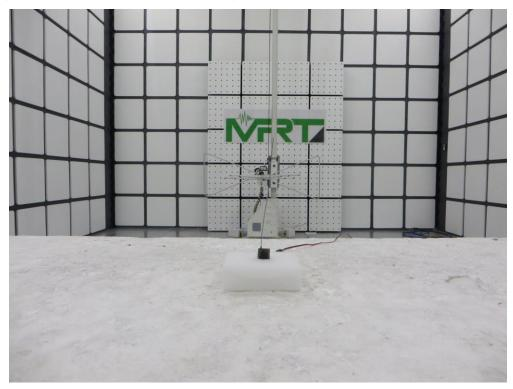
Description: Radiated Emission Test Setup for 1GHz ~ 18GHz (SPM9746) (1.5m Height)
