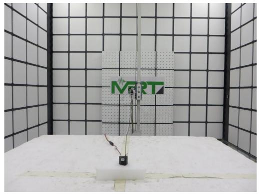
Description: Radiated Emission Test Setup for 9kHz ~ 30MHz (SPM9746) (0.8m Height)
