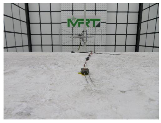
Description: Radiated Emission Test Setup for  $1GHz \sim 18GHz$
