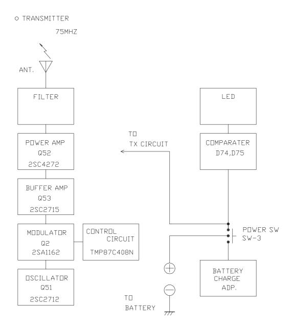
FCC ID# BRWPYTHON Figure 5.1 Transmitter Block Diagram
