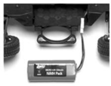
Plug the AC charger into the proper wall receptacle (110V - US version). Plug the battery pack into the charger and let it charge for 1 hour for the first time. Charge for 1 hour thereafter for a full charge. Battery charged for over 1 hour may cause an overcharge.
