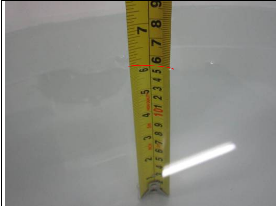
Liquid depth \geq 15cm
