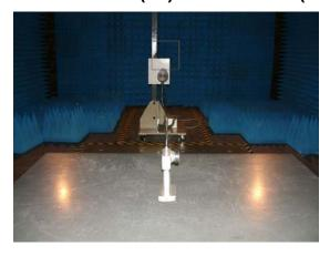
Photos of Radiated emission (TX) measurement (Above 30MHz)
