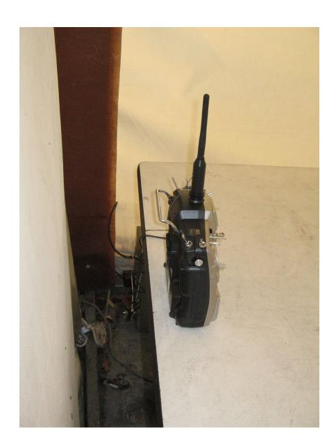
Photo showing connection of EUT rf port to antenna in host fixture.
