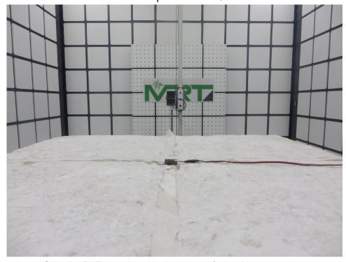
Note: For above 1GHz, the EUT was placed in the centre of turntable.
