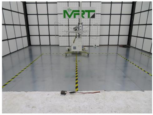
Note: For below 1GHz, the EUT was placed in the centre of turntable, and the edge of the test table is aligned with the diameter of the turntable.
