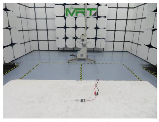
Description: Radiated Emission Test Setup for 1GHz ~ 18GHz
