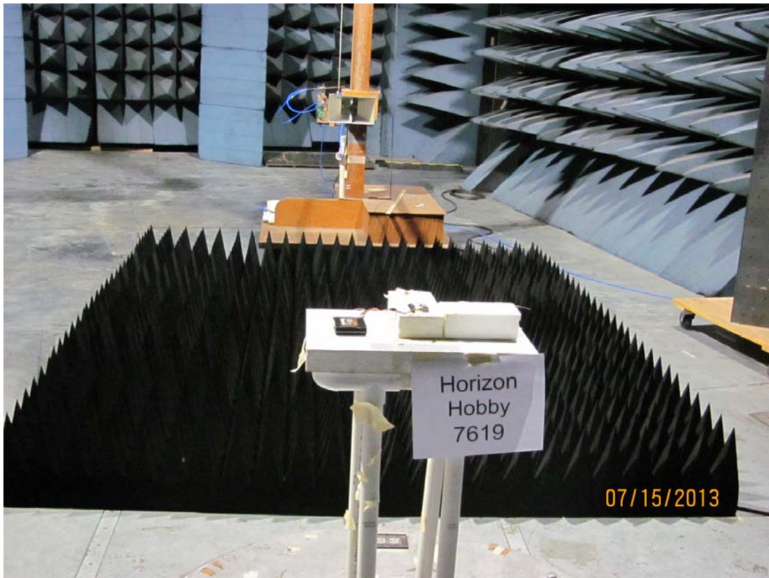
Photograph of Antenna Conducted Emissions Test Setup
