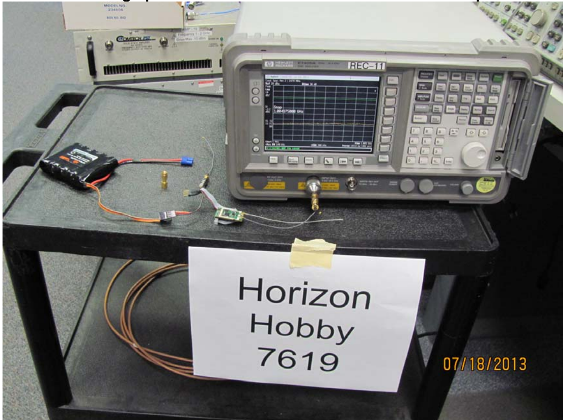
Photograph of Antenna Conducted Emissions Test Setup
