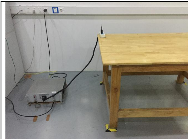
Conducted Emissions Test Setup – Front View
