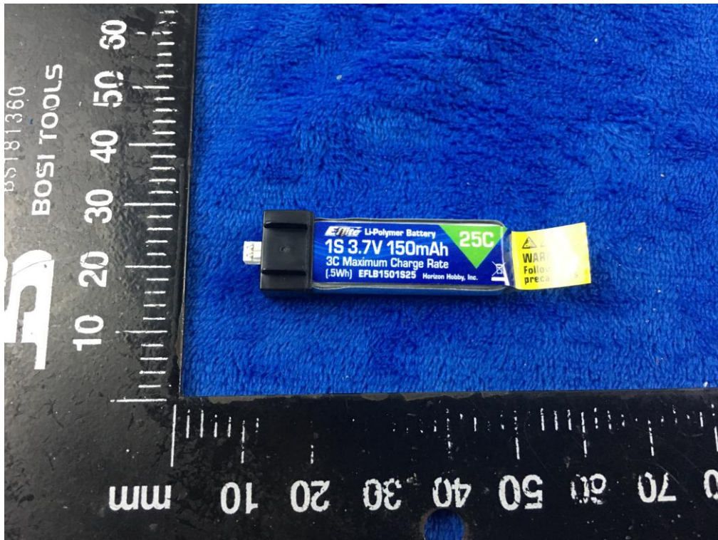
Battery - Front View
