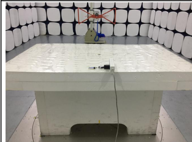
Radiated Emissions Test Setup Below 1GHz
