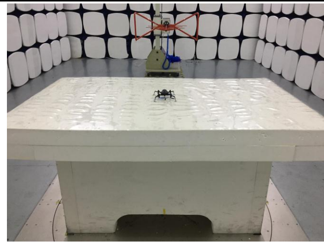
Radiated Spurious Emissions Test Setup Below 1GHz
